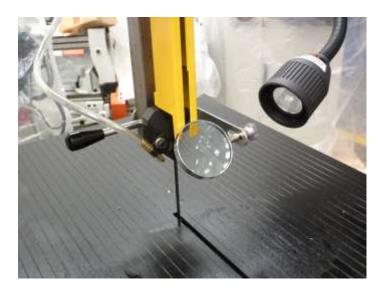
Magnifier, flexi-light and air deflector all located close to the blade for ease of operation.
