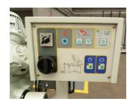
Electronic control panel, troubleshooting display. Semi-automatic operation, single button commences cycles, vice clamp, bow descends to perform cut, at finish of cut bow returns, vices unclamp.
