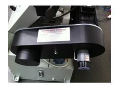
Heavy Duty 3 phase motor. Easy to change infinitely variable blade speed gearbox.
